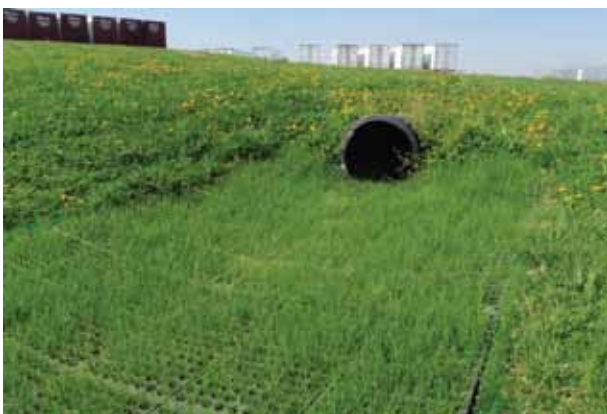
ShoreMax transition mats facilitate vegetation growth through voids in the mat and are a smart option to replace rock in high scour areas such as pipe outlets.
